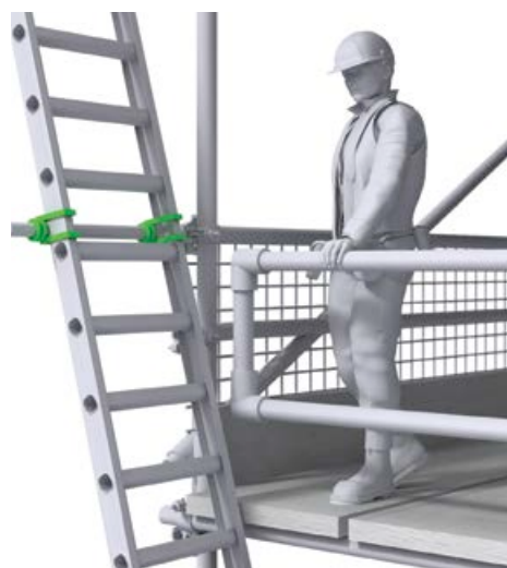
✓ Figure 9 Correct – access ladders should be tied and extend at least 1 m above the landing point to provide a secure handhold
