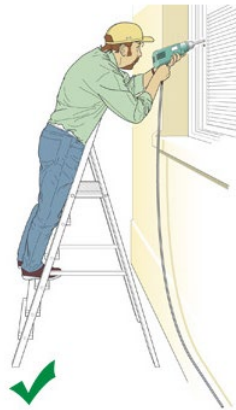
Correct Steps facing work activity.
